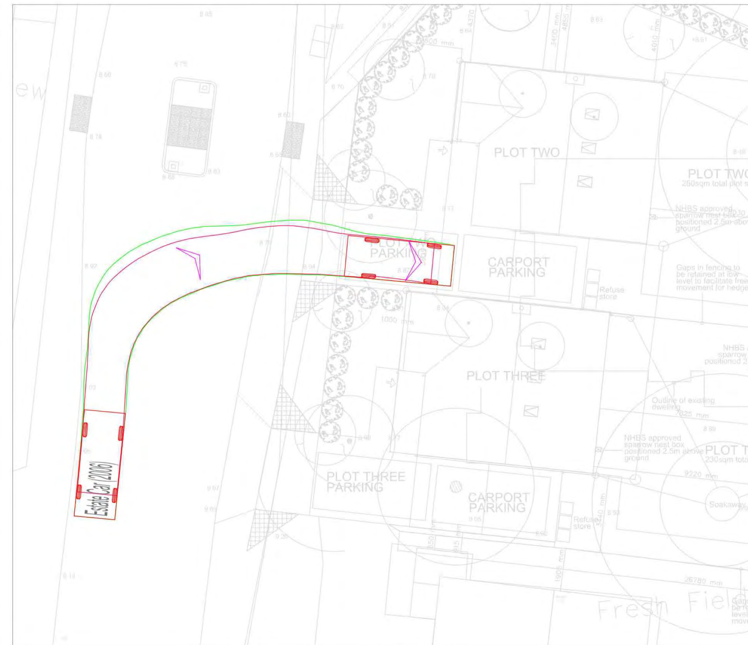
Swept Path - In - Forwards Direction Far side
